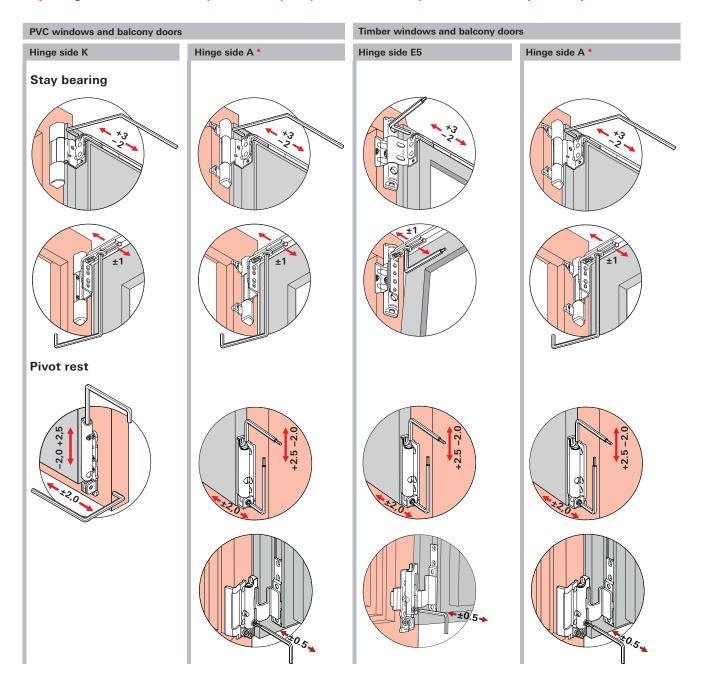
\*The indicated adjusting dimensions change upon use of cover caps (on stay bearing / pivot rest) and corner-rebate-security components.
